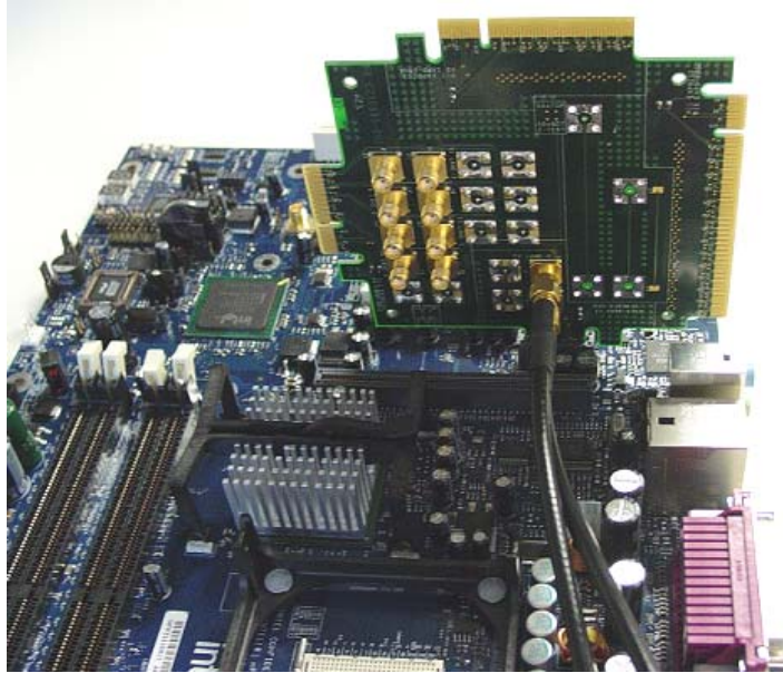
Figure 22 Connecting the PCI Express Signal Quality Test Fixture
